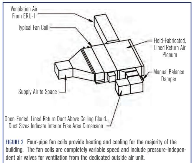
FIGURE 2 Four-pipe fan coils provide heating and cooling for the majority of the building. The fan coils are completely variable speed and include pressure-independent air valves for ventilation from the dedicated outside air unit.
