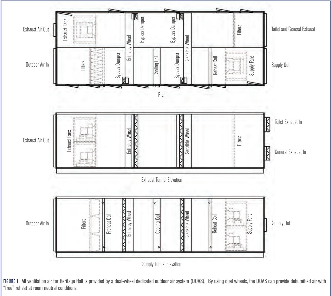
FIGURE 1 All ventilation air for Heritage Hall is provided by a dual-wheel dedicated outdoor air system (DOAS). By using dual wheels, the DOAS can provide dehumidified air with “free” reheat at room neutral conditions.
